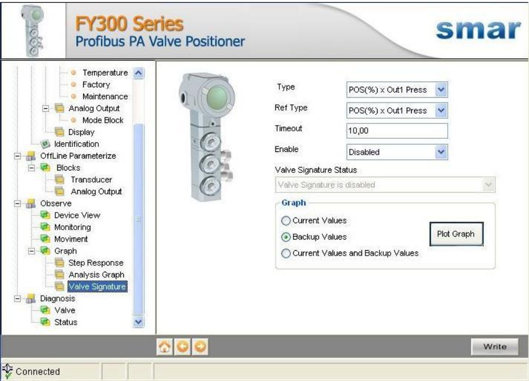
Figura 3.61 - Tela Inicial do Valve Signature
