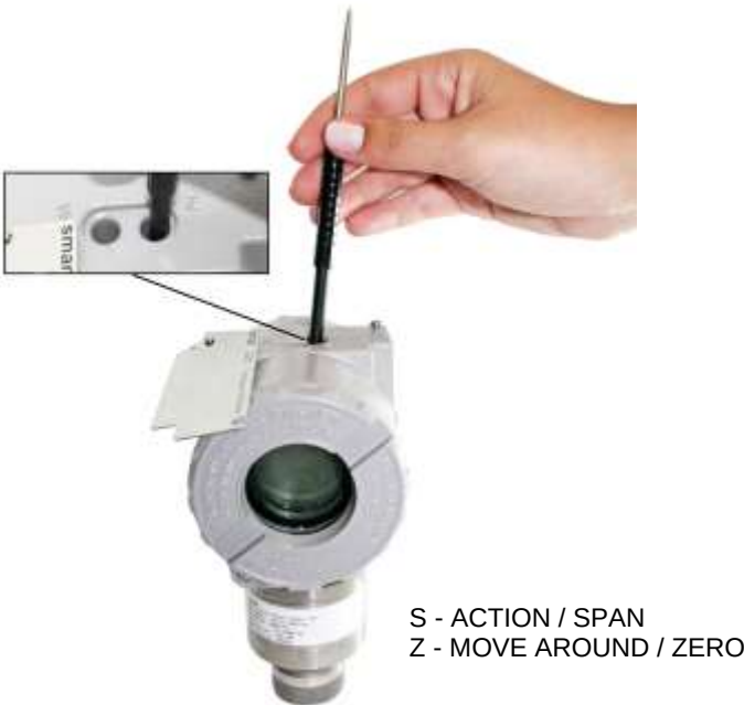
Figure 4.1 – Local Zero and Span Adjustment and Local Adjustment Switches
